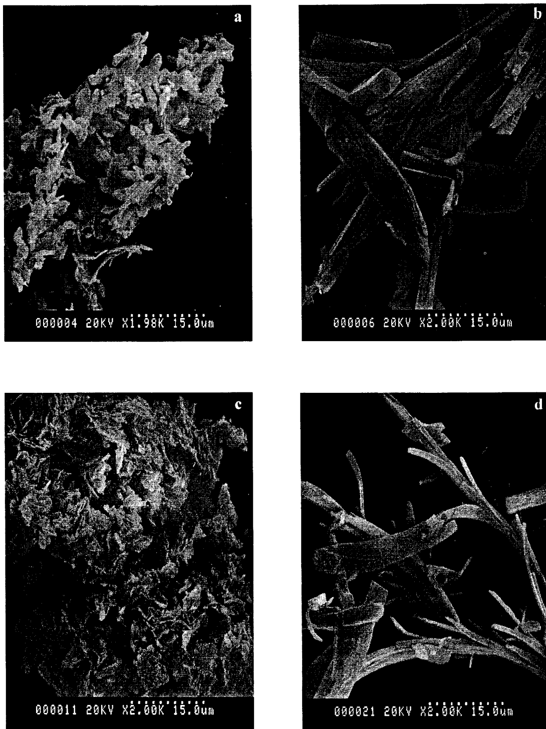
Fig. 6. Scanning electron micrographs of the SEDS processed lactose samples. Process conditions: temperature = 90°C, lactose concentration = 10% w/v in water; flow rate of solution = 0.035 ml/min; flow rate of methanol = 0.665 ml/min; (a) pressure = 150 bar, flow rate of liquid CO 2 = 19.0 ml/min; (b) pressure = 150 bar, flow rate of liquid CO 2 = 5.0 ml/min (c) pressure = 300 bar, flow rate of liquid CO 2 = 19.0 ml/min (d) pressure = 300 bar, flow rate of liquid CO 2 = 5.0 ml/min.
